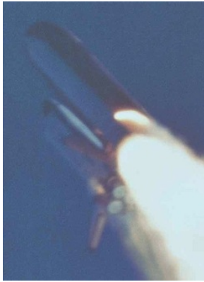
A NASA photograph showing the plume of flame from the side of the booster rocket during the Challenger launch.
